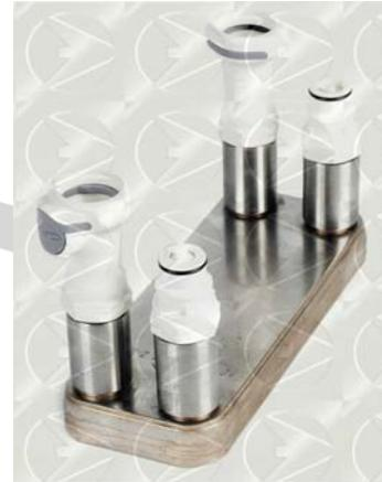
Multiple brazed stainless steel plates arranged for multi-pass operation with passes in series give a total heat transfer area of approximately 24000mm<sup>2</sup>. Four thermocouples measure hot and cold fluid entry and exit temperatures. Self sealing quick release connections enable rapid connection to the H102 and conversion from parallel to counter-current flow. **An extended version with intermediate measuring points and a total of 6 thermocouples is available as H102F.**
