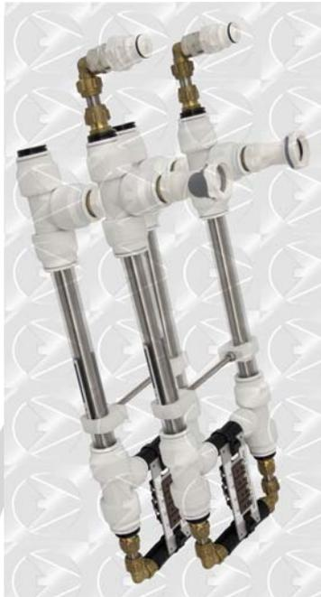
An extended version of the H102A Concentric Tube Heat Exchanger with 3 pairs of intermediate points giving 10 thermocouples in total. In conjunction with the H102A this allows investigation of the effects of increased heat transfer area and the plotting of more points on the temperature distribution graph.
