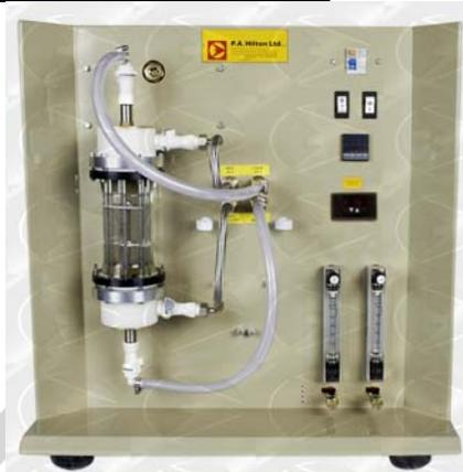
A bench mounted, reinforced plastic panel with an integral electrical console that provides services for any of the optional heat exchangers.
