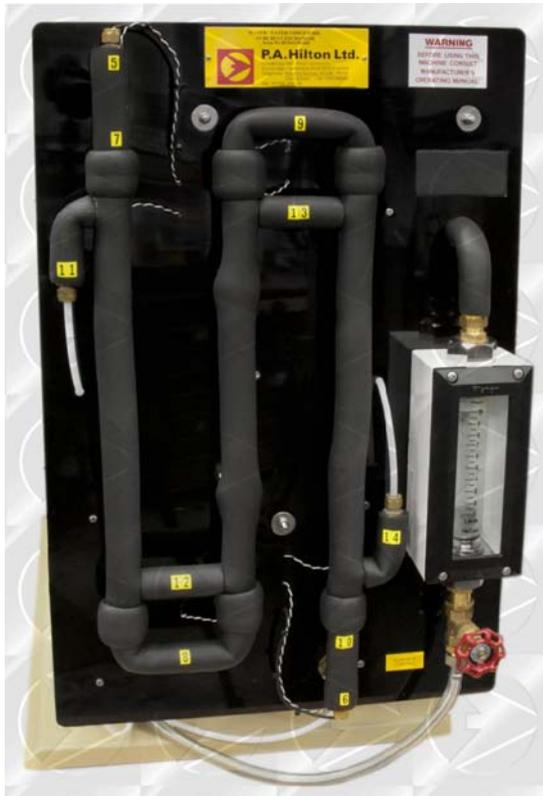
This is a highly advanced concentric tube heat exchanger with hot water flowing through the central tube while cooling water flows through the annular space.
