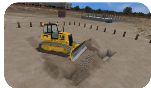
Using the blade to backfill a trench
