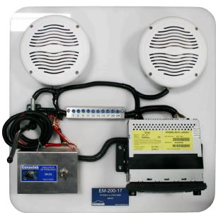
The ConsuLab EM-200-17 Audio System Trainer is mounted on a plastic training board with OEM components. It contains the following features:
