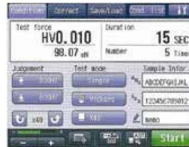
In standard test mode, test can be performed by setting detailed conditions such as sample information, shape corrections, and pass/fail determinations. Fracture toughness tests are also possible.
