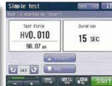
Simple test mode can be selected to start testing immediately just by setting the test force and the duration time.
