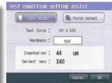
The system is equipped with a test conditions assist function to determine the optimal lens or test force from the estimated hardness.
