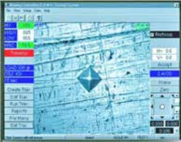
In recent years, instruments have been increasingly used by inexperienced operators. At the same time, reliable measurements are essential in order to ensure quality, so instruments are needed that can be used easily by anyone, with minimal risk of human measurement error. Our Micro Vickers Hardness Testers, featuring automatic length measurement, have been standardized as a response to such demands.
